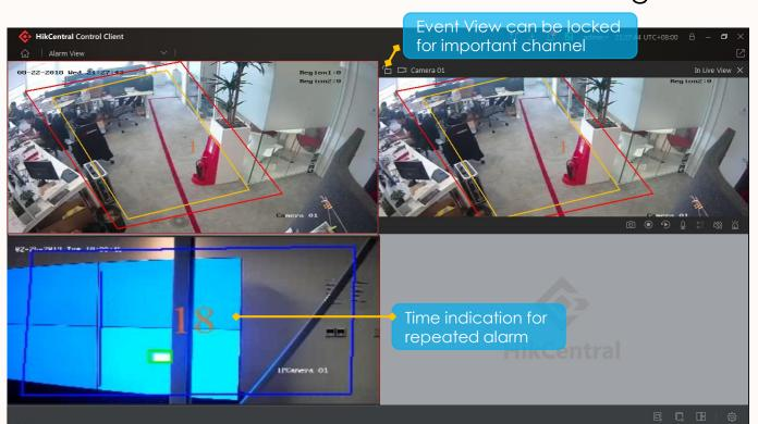
◆ For an alarm event which has been triggered continuously, it dwells on the same window with the repeated alarm times information indication.
