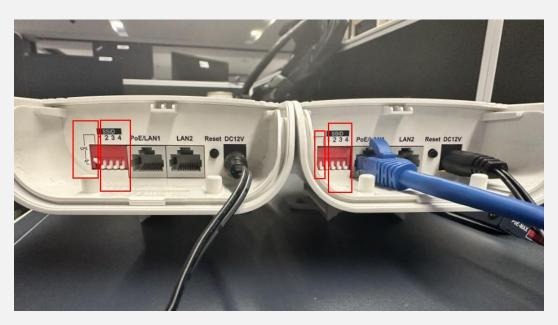
Besides this way, it supports to set the SSID by manual. Quit the Enable DIP Switch, and then input the name of SSID.
