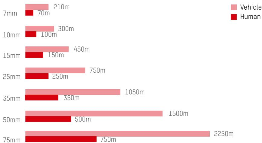
Notice: this distance is based on 17µm sensor.
