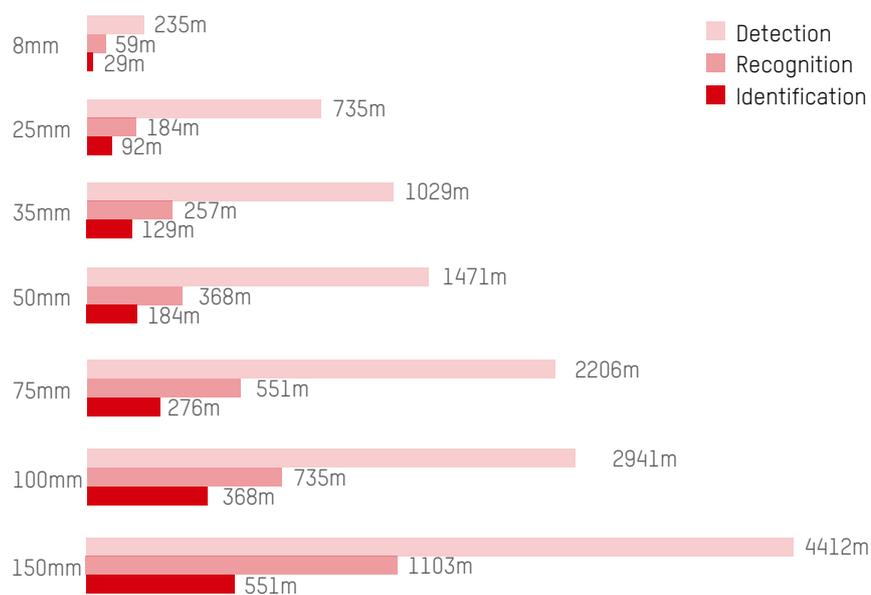
Notice: this distance is based on 17µm sensor
