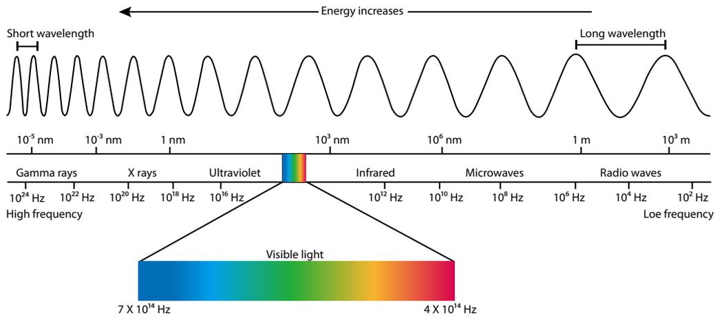
While invisible to human eyes, thermal cameras detect this kind of radiation (from wavelength 8 to 14  $\mu\text{m}$ , or 8,000 – 14,000 nm) and produce images (thermograms) using temperature differences. Thermography makes it possible to see the environment with or without visible light, and thus is widely used in such areas as video surveillance, fire detection, environmental control, building analyses, medical analyses, and others.
